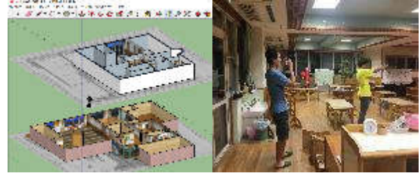
Figure 6: Three-dimensional data in SketchUp (left). We take photos of the interior of the nursery school to be used as a texture of the model (right).
